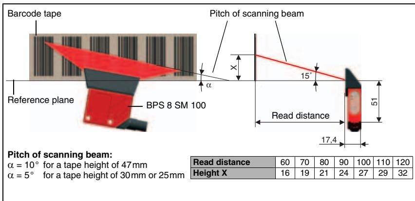
Figure 3.2: Beam exit and device arrangement for the BPS 8 SM 100
