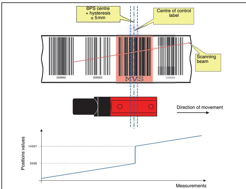
Figure 6.9: Switching position with the "MVS" control barcode
