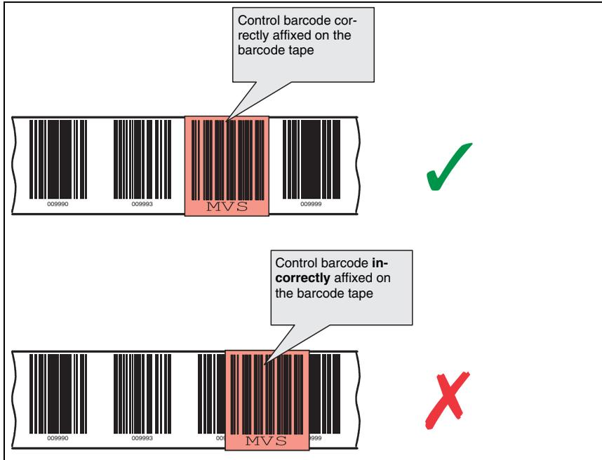
Figure 6.7: Correct positioning of the control barcode
