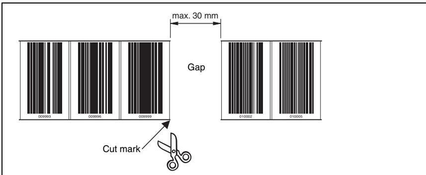
Figure 6.4: Gap in the cut barcode tape
