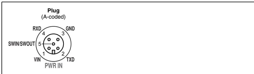
Figure 3.3: BPS 8 - assignment M12 connector PWR IN
