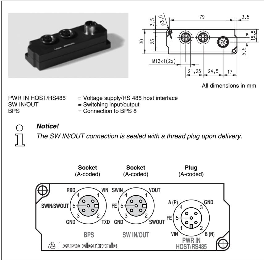
Figure 4.4: Connection assignment MA 8-01
