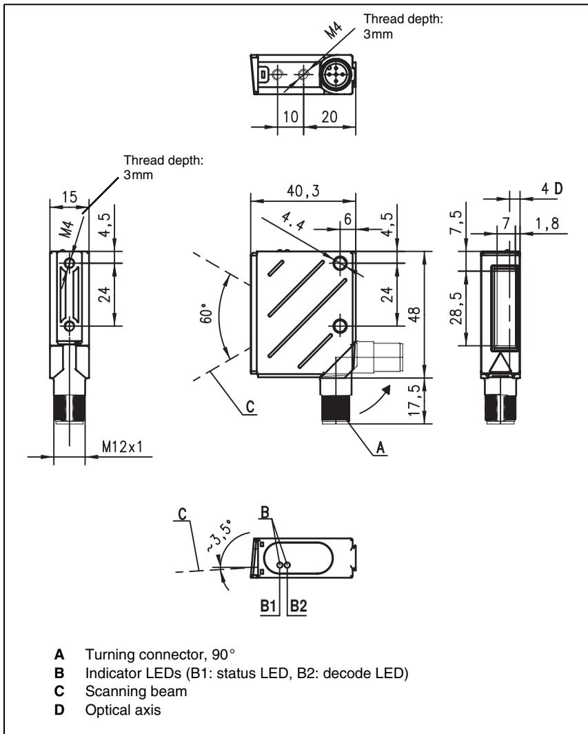
Figure 4.2: Dimensioned drawing BPS 8 SM 102-01
