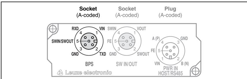
Figure 3.6: BPS 8 - Connection to the MA 8-01
