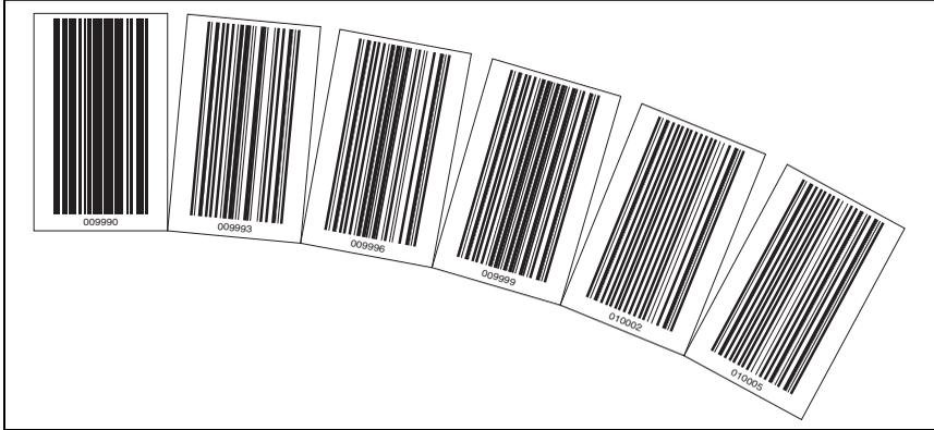
Figure 6.5: Partial cutting of the barcode tape in curves
