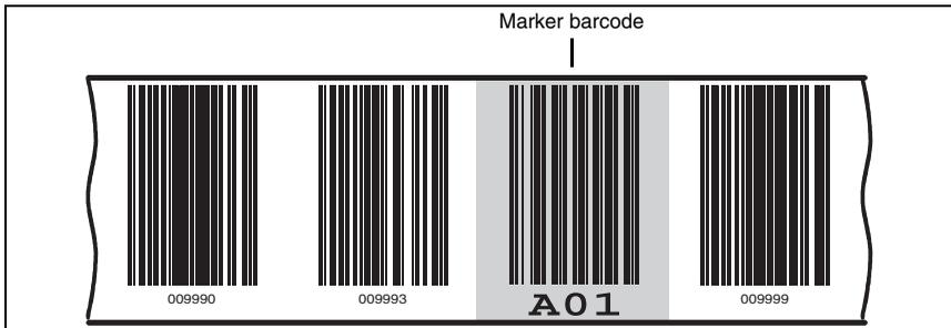
Figure 9.4: System arrangement of marker labels
